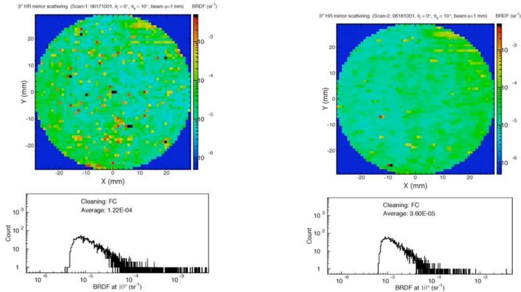
On the left is the same optic as was used above for the clear first contact tests. It sat around collecting big dust particles for a couple weeks in the CASI system, which resulted in an average BRDF of  $1.22 \times 10^{-4}$ . On the right is the BRDF after cleaning it with red First Contact, its average value was  $3.6 \times 10^{-5}$ .
