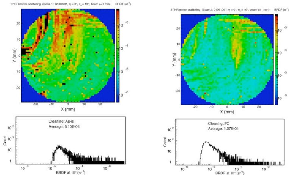
On the left is a scan of an optic before it was cleaned. The average brdf value is  $6.10 \times 10^{-4}$ . On the right is the same optic after it was cleaned once with clear first contact, it's average value is  $1.07 \times 10^{-4}$ . Successive cleanings with clear first contact seemed to improve the BRDF at around the same rate.
