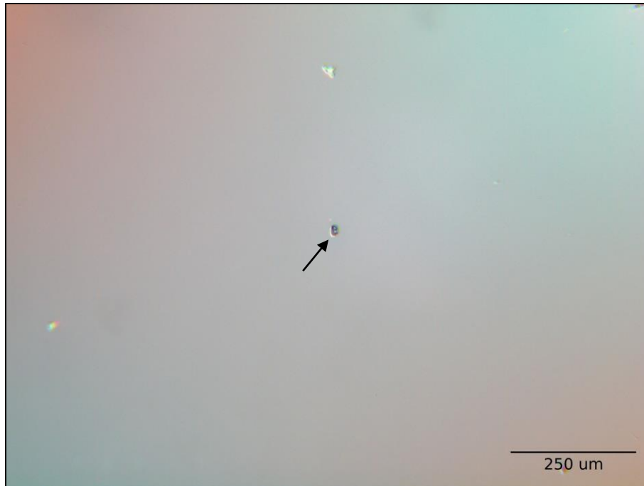
Fig. 5 Typical polarizing surface damage morphology (P pol.) (Fluence 4.00 J/cm 2 , damage after 2 pulses)
