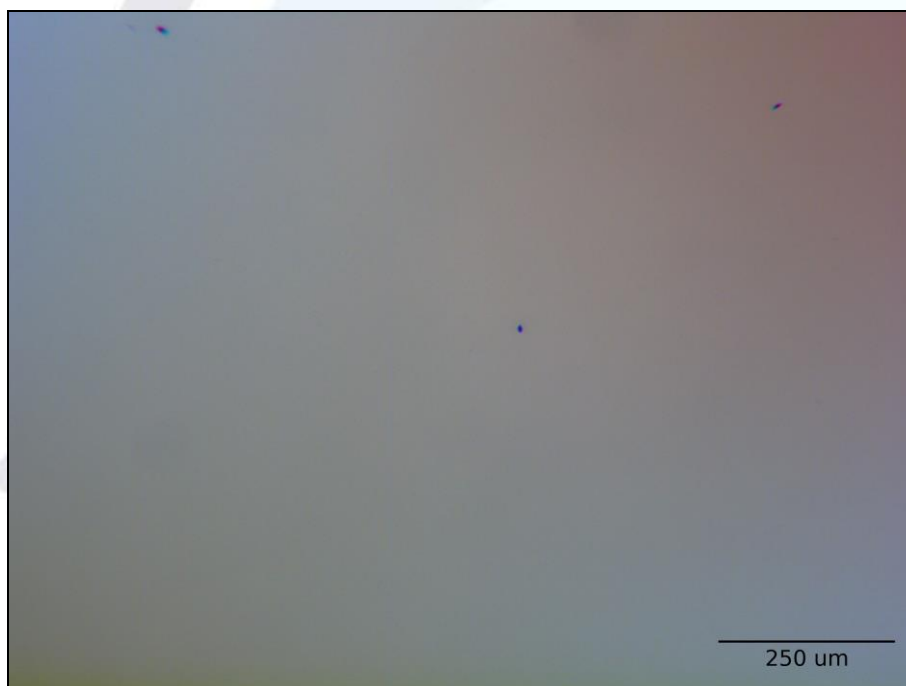
Fig. 6 Typical polarizing surface damage morphology (P pol.) (Fluence 3.14 \text{ J/cm}^2 , damage after 69 pulses)
