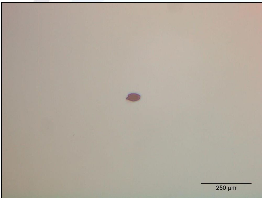
Fig. 4 Typical front surface damage morphology (Energy density 25.98 J/cm 2 , damage after 1000 pulses)
