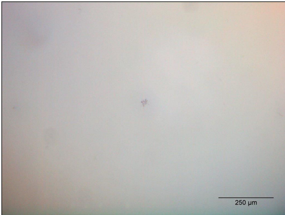
Fig. 3 Typical front surface damage morphology (Energy density 5.34 J/cm 2 , damage after 1 pulse)
