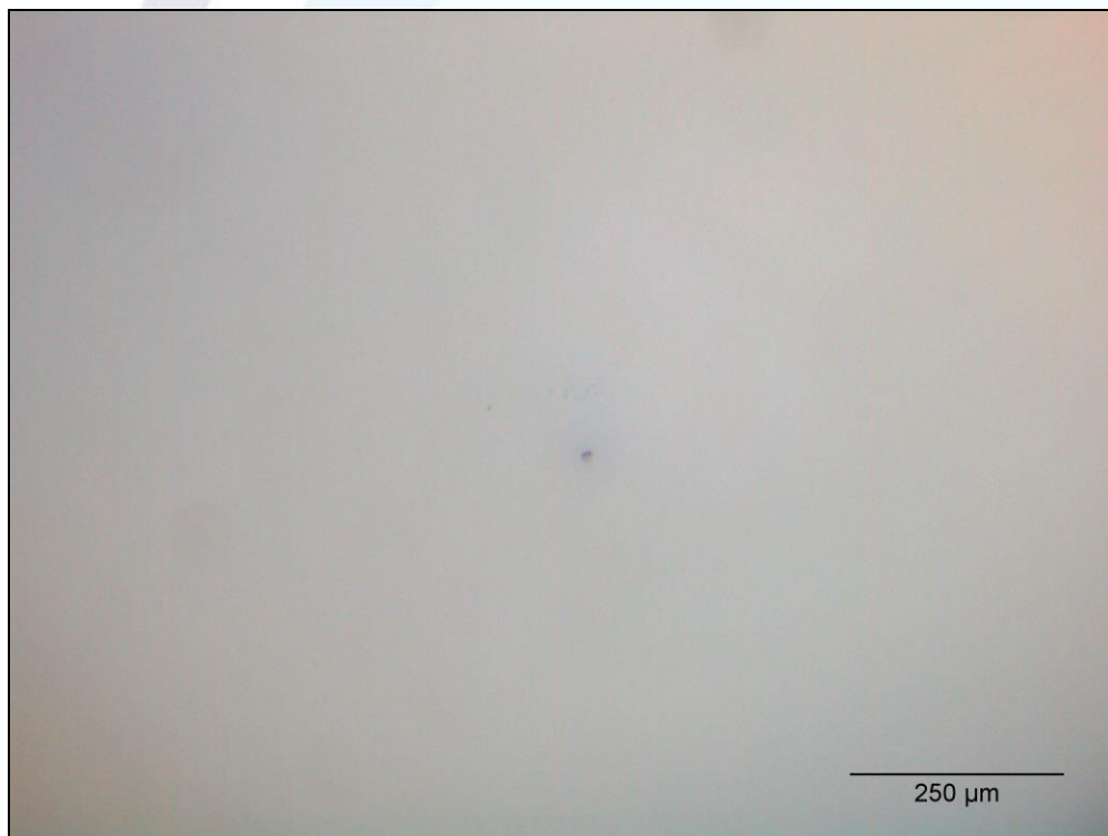
Fig. 4 Typical in volume damage morphology (Energy density 19.97 J/cm 2 , damage after 263 pulses)
