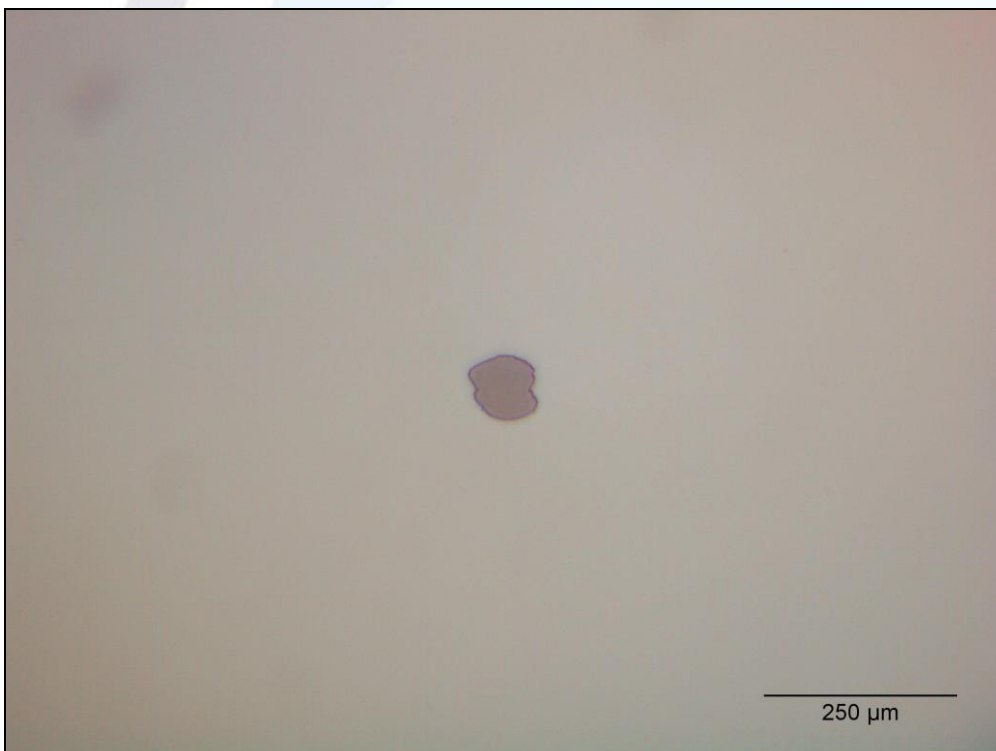
Fig. 4 Typical front surface damage morphology (Energy density 26.00 J/cm 2 , damage after 1000 pulses)
