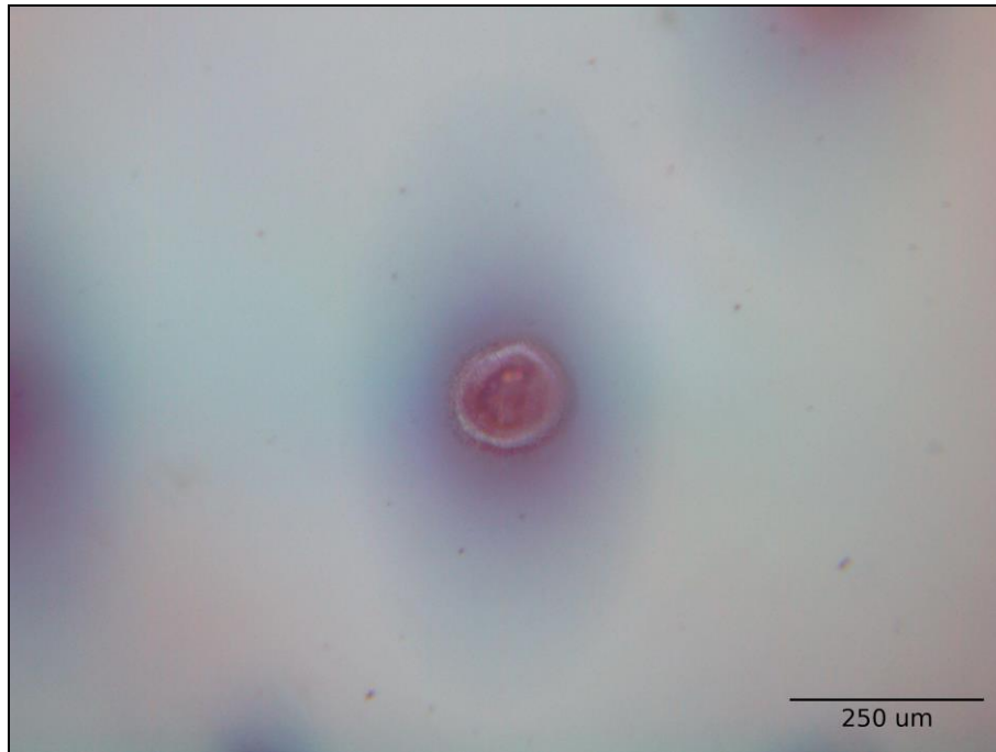
Fig. 5 Typical front surface damage morphology (P pol.) (Fluence 6.61 \text{ J/cm}^2 , damage after 12 pulses)
