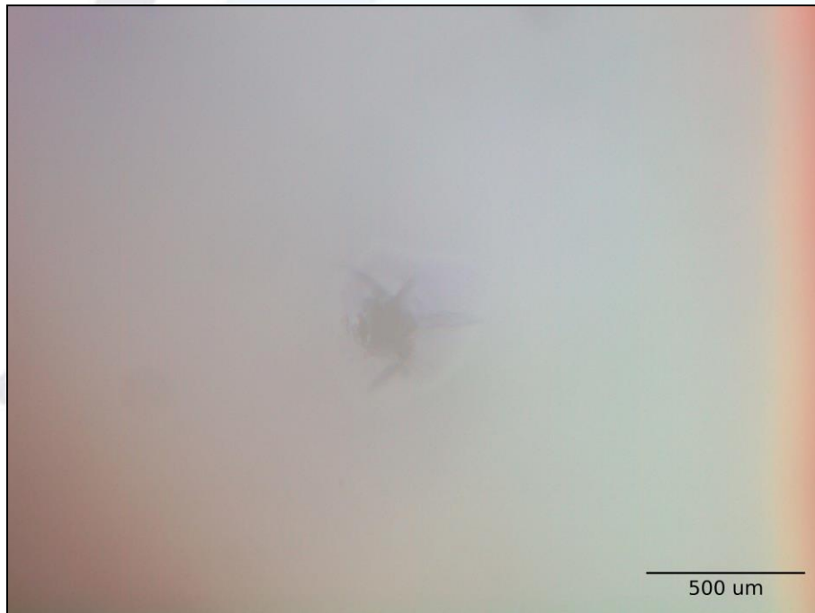
Fig. 4 Typical polarizing surface damage morphology (Fluence 31.7 J/cm 2 , damage after 5 pulses)
