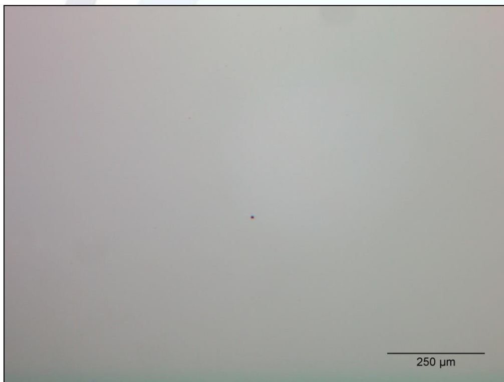
Fig. 4 Typical damage morphology (Fluence 0.70 J/cm 2 , damage after 255 pulses)
