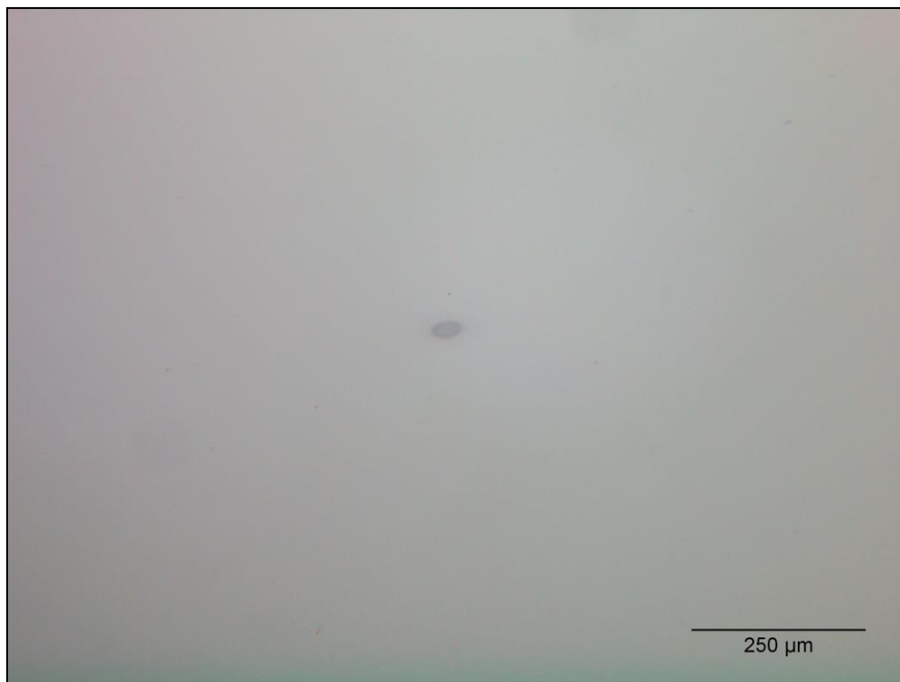
Fig. 3 Typical damage morphology (Fluence 1.26 J/cm 2 , damage after 1 pulse)
