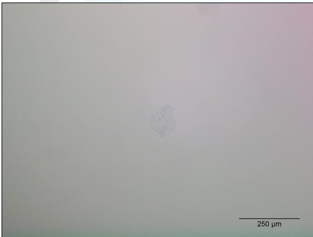
Fig. 4 Typical damage morphology (Fluence 2.52 J/cm 2 , damage after 1000 pulses)
