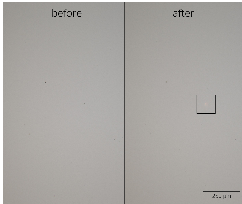
Figure 4. Typical damage morphology: fluence 13.7 J/cm 2 , damage after 1000 pulse(s).
