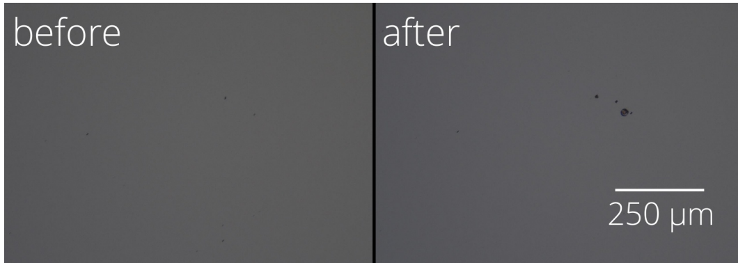
Figure 4. Typical damage morphology: fluence 47.3 J/cm 2 , damage after 1 pulse(s).
