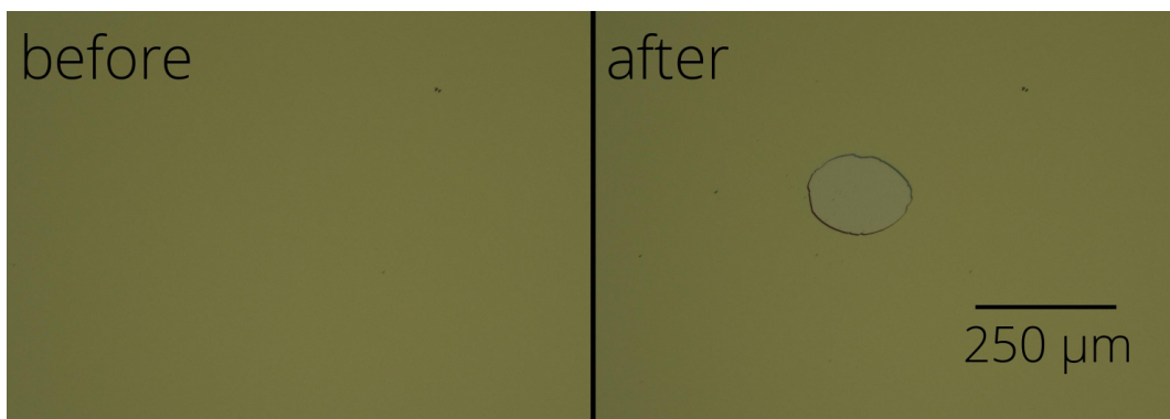
Figure 6. Typical damage morphology: fluence 47.1 J/cm 2 , damage after 67 pulse(s).
