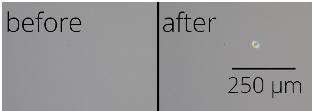
Figure 4. Typical damage morphology: fluence 16.3 J/cm 2 , damage after 1000 pulse(s).
