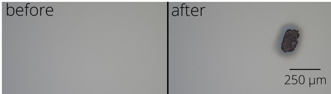
Figure 4. Typical damage morphology: fluence 4.73 \text{ J/cm}^2 , damage after 222 pulse(s).
