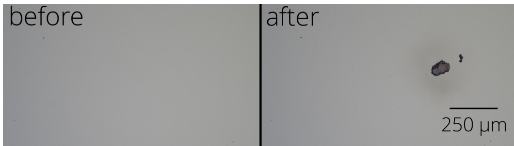
Figure 5. Typical damage morphology: fluence 6.19 \text{ J/cm}^2 , damage after 10 pulse(s).
