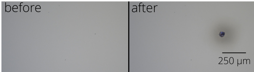
Figure 4. Typical damage morphology: fluence 3.96 \text{ J/cm}^2 , damage after 176 pulse(s).
