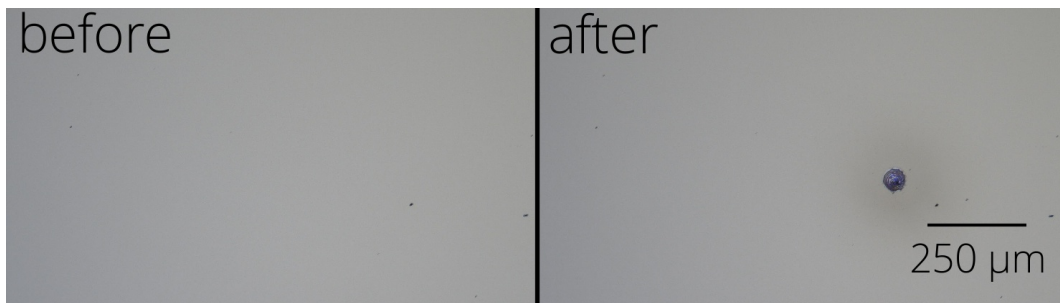
Figure 5. Typical damage morphology: fluence 5.56 \text{ J/cm}^2 , damage after 69 pulse(s).
