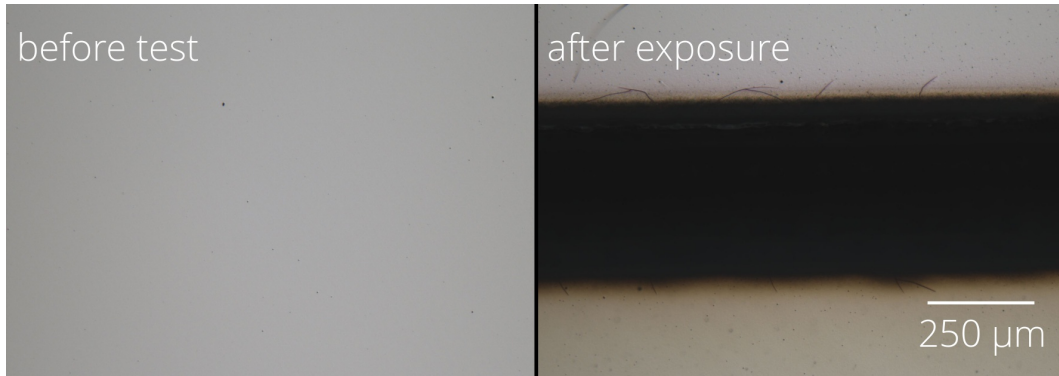
Figure 7. Typical damage morphology: irradiance 0.198 \text{ MW/cm}^2 .
