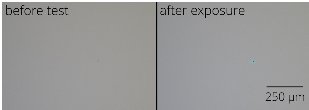
Figure 4. Typical damage morphology: fluence 3.54 \text{ J/cm}^2 , damage after 698 pulse(s).
