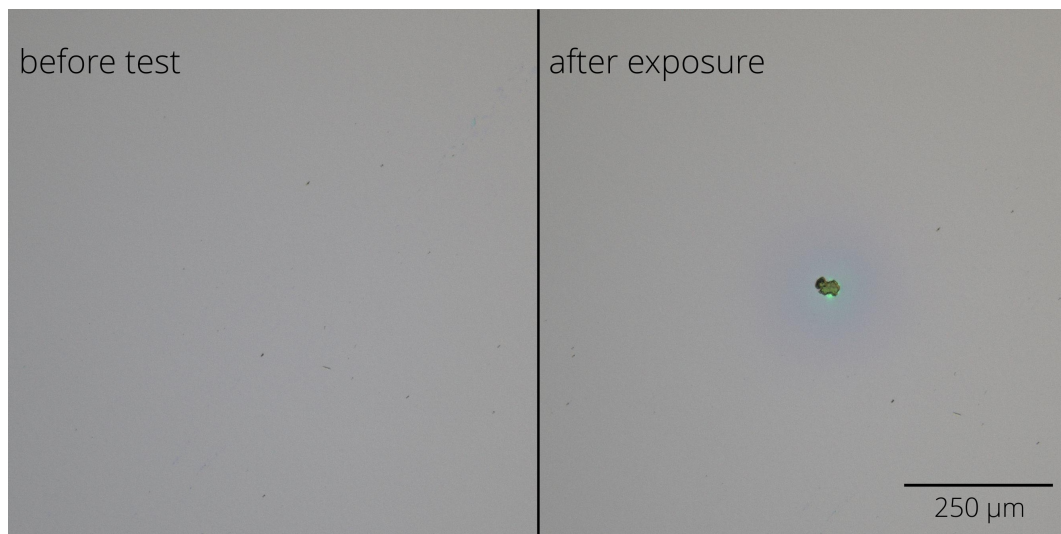
Figure 5. Typical damage morphology: fluence 19.9 J/cm 2 , damage after 15 pulse(s).
